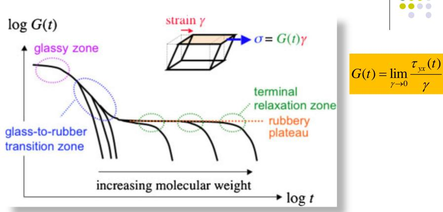
Viscoelastic relaxation modulus of flexible linear polymers.
