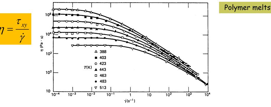
Viscosity of LDPE melts at various temperatures
