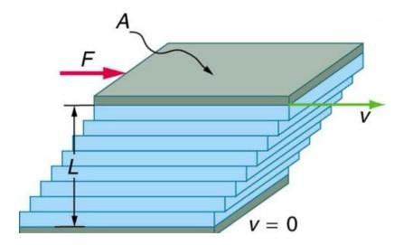
Startup of Steady Shear Flow or Stress Growth
