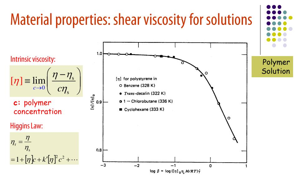
The intrinsic viscosity **[n]** of polystyrene in various solvents, as a function of a normalized rate of deformation,  $\beta$ . [n]<sub>o</sub>: zero shear value, n<sub>s</sub> solvent viscosity.
