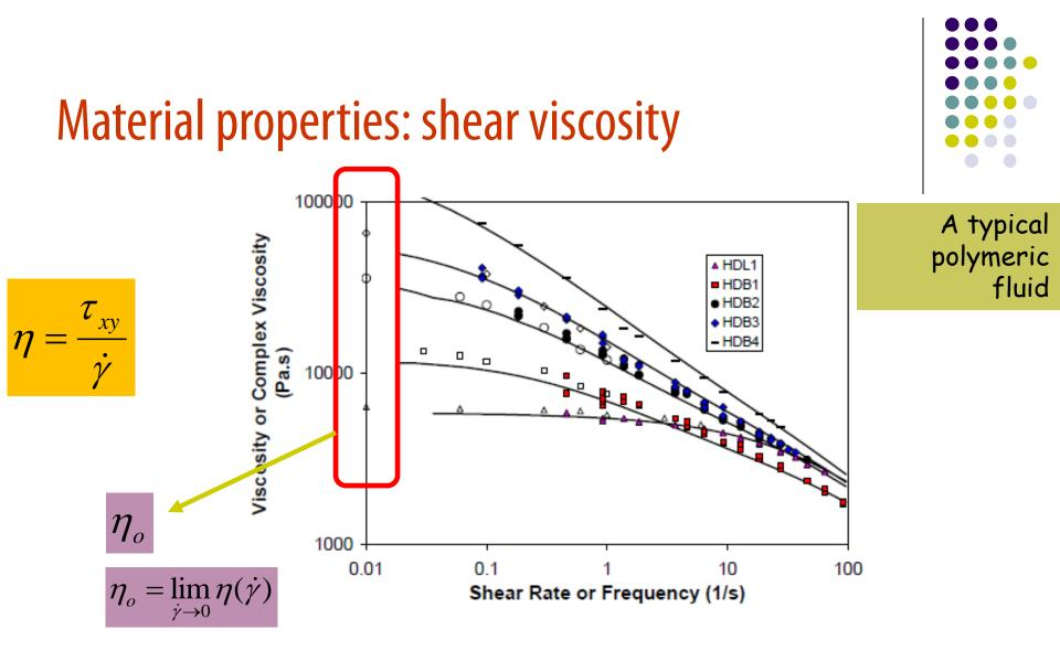
At low shear rates the viscosity is independent of the shear rate. It is called zero shear rate viscosity  $n_0$ .
