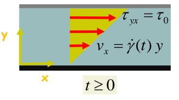
7. Constrained Recoil after steady Shear Flow
